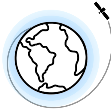
Figure 4.15: A diagram illustrating how the force of drag slows down a satellite, causing an eventual deorbit.
